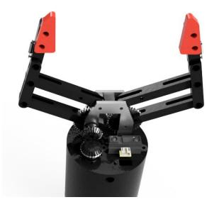
The fingers are mounted on a four-bar linkage, which provides a large range of motion without greatly increasing the size of the hand in the way that a rack and pinion or leadscrew would. A single motor drives both linkages, with spur gears transmitting power between them. Using a single motor reduces component cost, space usage, and overall system complexity.
